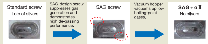
Resin: PC not processed with dryer * SAG + α II requires a SAG screw and a vacuuming-applicable heat barrel in addition to the vacuum hopper. * Products, resins and mold structures affect the performance of SAG + α II.
